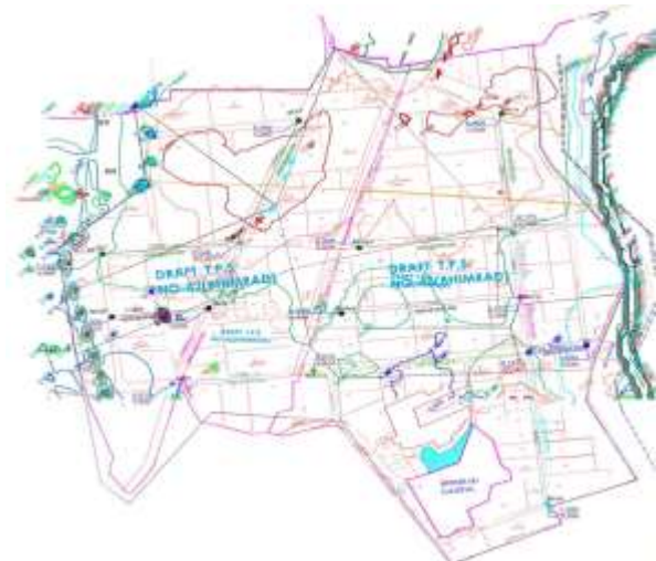
Storm water drainage network derived from DEM
